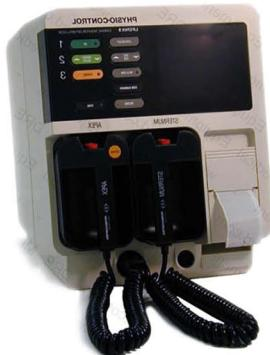
The Lifepak 9 is defibrillator/monitor,cardioscope and non-invasive pacemaker. It provides 17 energy selections, heart rate alarms, three-lead ECG monitoring, recorder and Code Summary™ critical event recorder.
